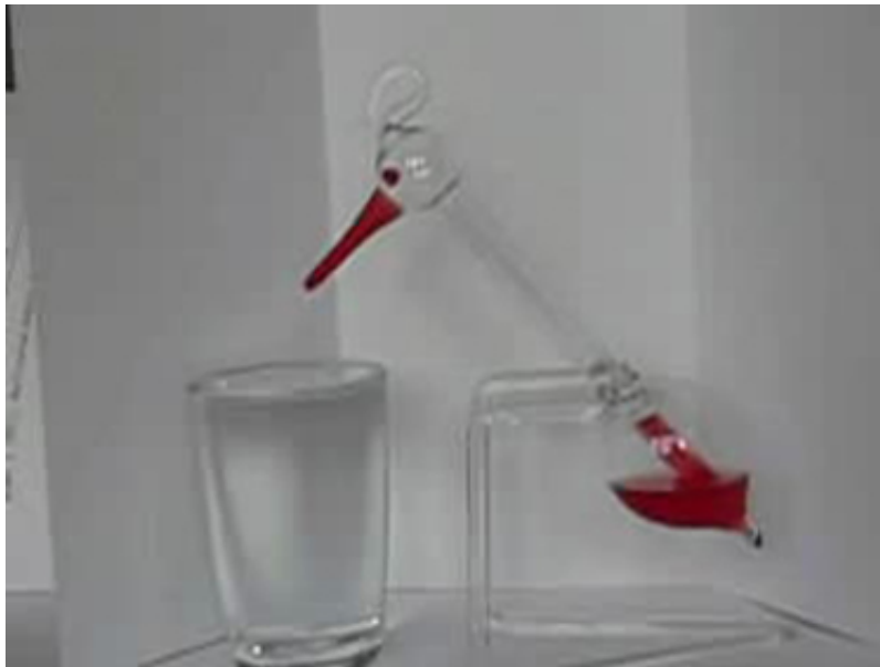
Figure 15.21 This novelty toy, known as the drinking bird, is an example of Carnot's engine. It contains methylene chloride (mixed with a dye) in the abdomen, which boils at a very low temperature—about 100°F. To operate, one gets the bird's head wet. As the water evaporates, fluid moves up into the head, causing the bird to become top-heavy and dip forward back into the water. This cools down the methylene chloride in the head, and it moves back into the abdomen, causing the bird to become bottom heavy and tip up. Except for a very small input of energy—the original head-wetting—the bird becomes a perpetual motion machine of sorts. (credit: Arabesk.nl, Wikimedia Commons)
